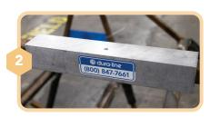
Slide the gauge over the damaged spoke. If the gauge cannot slide along the spoke, the reel is too damaged to be accepted.
