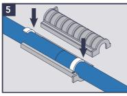
Place the top of the connector into position.
