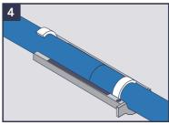
Clip the second duct into place and visually check that the seal has not been displaced. Ensure the cable is straight.
