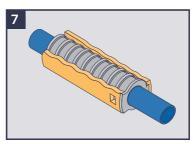
Tap them with a soft mallet until the end of the clasp is level with the end of the connector.
