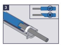
Clip one duct into the white grip ring that is attached to the connector. Ensure that the ends of the duct are cut square.
