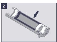
Apply silicone grease along both rubber seals, ensuring the surface areas of the seals are completely covered.
