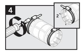
Loosen the band clamps to allow spreading of the split segments on the end of the coupler during insertion.
