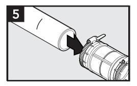
Push conduit into the coupler past the grip ring and O-ring until it hits the center stop and the mark is aligned with the end of the coupler. This ensures the O-ring is seated properly.
