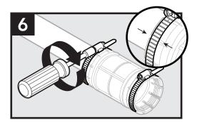
Verify the band clamp is positioned in the groove and fully tighten it down.
