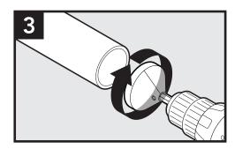
If possible, chamfer the leading edge of the conduit for smoother insertion.
