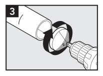
Chamfer the end to allow for smooth insertion.
