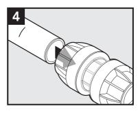
Do not unscrew Bell End. Push conduit into coupler to the mark to ensure O-ring is seated around the duct. The clear midsection allows for visual confirmation that duct is properly seated.
