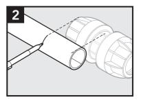
Align both ducts at the center of the coupler and mark ends.
