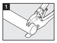
Cut conduit flush with duct cutters.
