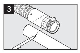
Overlap ends of conduit. Place duct at center of coupler and mark at the end.
