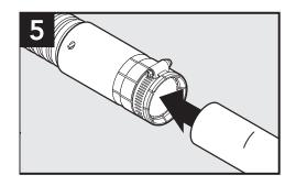
Push conduit into the coupler past the grip ring and O-ring until the mark is aligned with the end of the coupler. This ensures the O-ring is seated properly.
