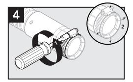
Loosen the band clamp to allow spreading of the split segments on the end of the coupler during insertion.
